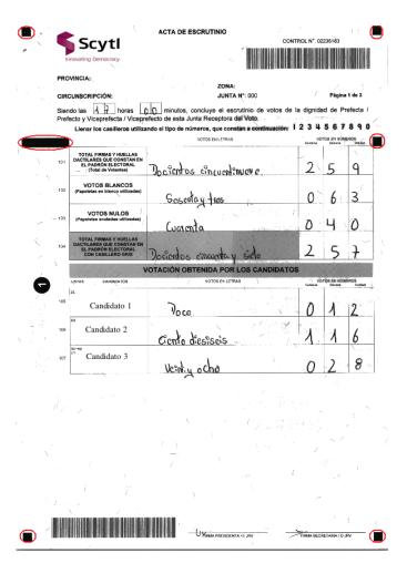
Fig. 2. The fiducial marks in a tally sheet (highlighted in red) used to detect the orientation and skew also allow us to segment the Region of Interest for later handwriting and digit recognition steps.
