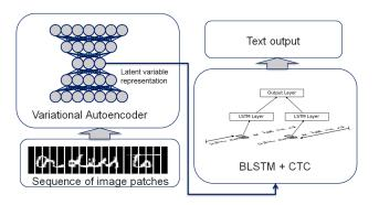
Fig. 3. A sequence of image patches is passed through the encoder of a Variational Autoencoder to get a latent variable representation. This representation is then fed into a bidirectional long short term memory neural network to perform the final recognition.
