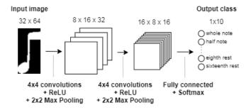
Fig. 1. Scheme of the architecture of the CNN we used. All convolutions are done with a padding of 2 to preserve the image size.
