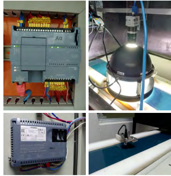
Figure 2: (top-left) Siemens S7 1200 PLC. (bottom-left) HMI TP700 comfort. (top-right) Vision system and lighting system. (bottom-right) Inductive Sensor.
