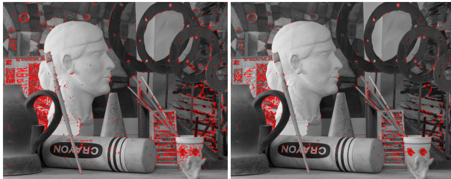
Fig. 2. Results from Harris algorithm with: ( left ) low threshold value and ( right ) high threshold value
