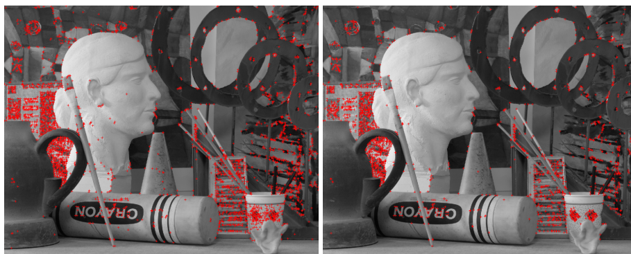
Fig. 4. Results by tuning Harris algorithm according to [9], considering 9 sub-images and setting: ( left ) p = 0.005 and ( right ) p = 0.015 respectively
