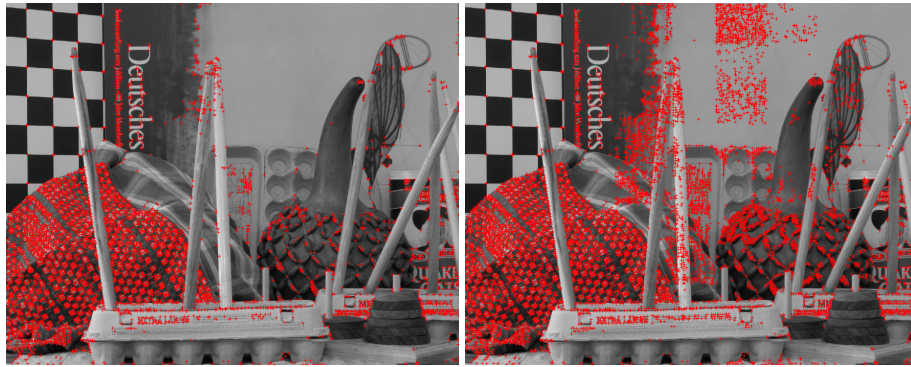
Fig. 5. Result by tuning Harris algorithm according to [9], setting p = 0.005 and considering: (left) 9 sub-images and (right) 81 sub-images respectively
