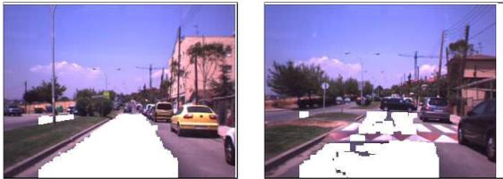
Fig. 3. Rapid road segmentation associated with two frames.
