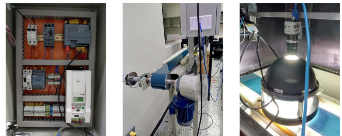
Fig. 3. (1st) Siemens S7 1200 PLC. (2nd) Conveyor belt. (3rd) Industrial camera and lighting system.
