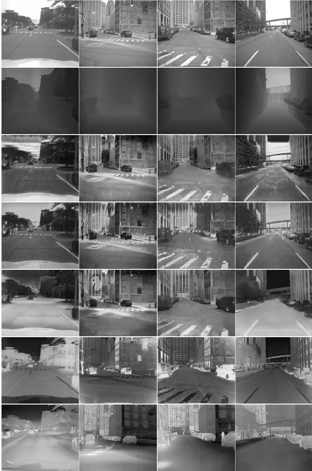
Fig. 4. Experimental results from FLIR ADAS V2 dataset: (1st. row) Brightness channel from the HSV representation; (2nd. row) Depth map obtained from [13]; (3rd. row) Thermal representation from [14]; (4th. row) Thermal representation from [18] (CUT); (5th. row) Thermal representation from [18] (FastCUT); (6th. row) Thermal representation from the proposed approach; (7th. row) Ground truth images.
