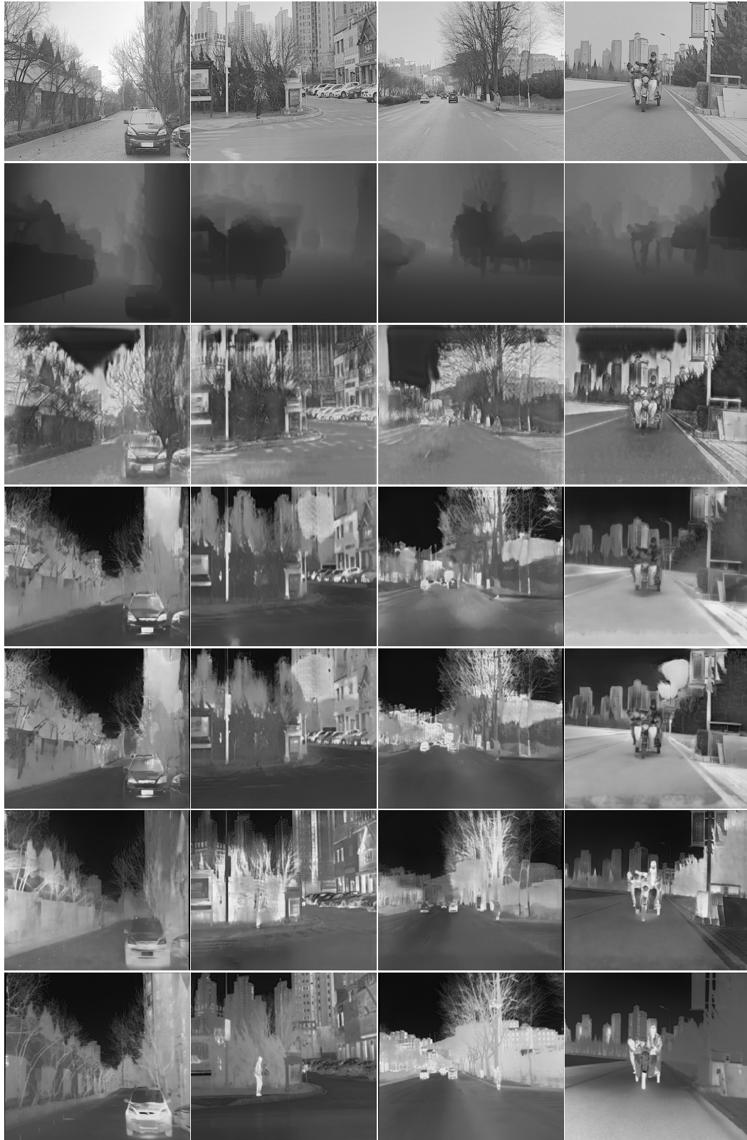
Fig. 2. Experimental results from M3FD dataset: (1st. row) Brightness channel from the HSV representation; (2nd. row) Depth map obtained from [13]; (3rd. row) Thermal representation from [14]; (4th. row) Thermal representation from [18] (FastCUT); (5th. row) Thermal representation from [18] (FastCUT); (6th. row) Thermal representation from the proposed approach; (7th. row) Ground truth images.
