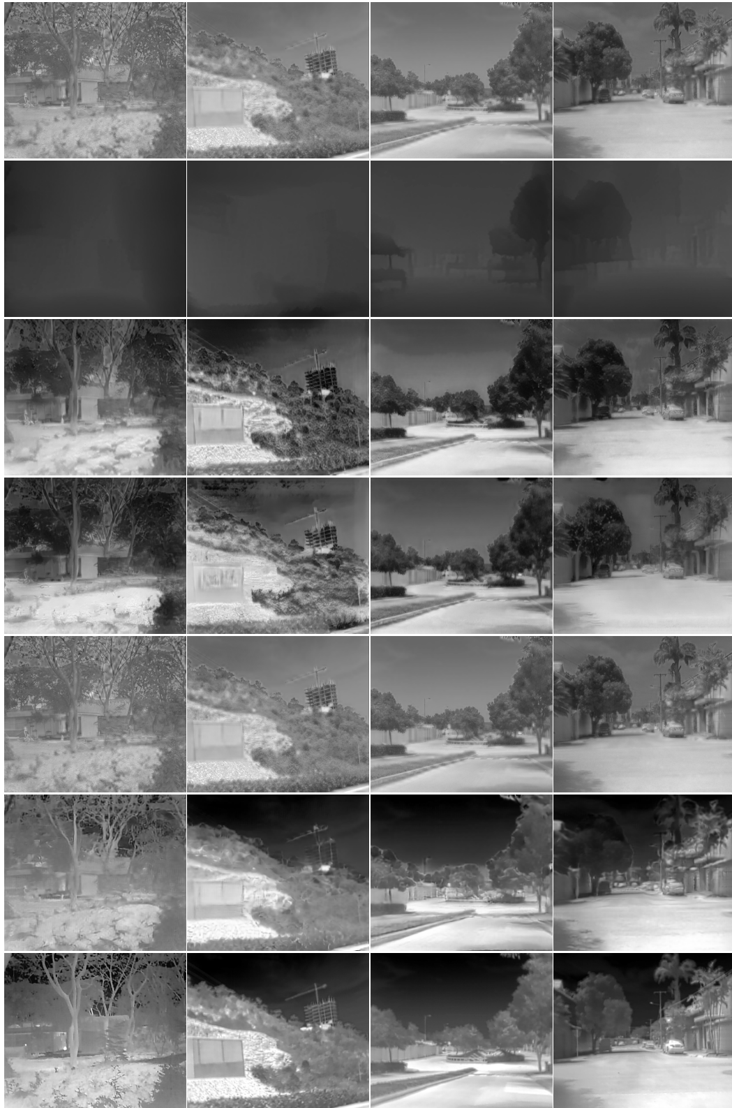
Fig. 3. Experimental results from Thermal Stereo dataset: ( 1st. row ) Brightness channel from the HSV representation; ( 2nd. row ) Depth map obtained from [13]; ( 3rd. row ) Thermal representation from [14]; ( 4th. row ) Thermal representation from [18] (CUT); ( 5th. row ) Thermal representation from [18] (FastCUT); ( 6th. row ) Thermal representation from the proposed approach; ( 7th. row ) Ground truth images.
