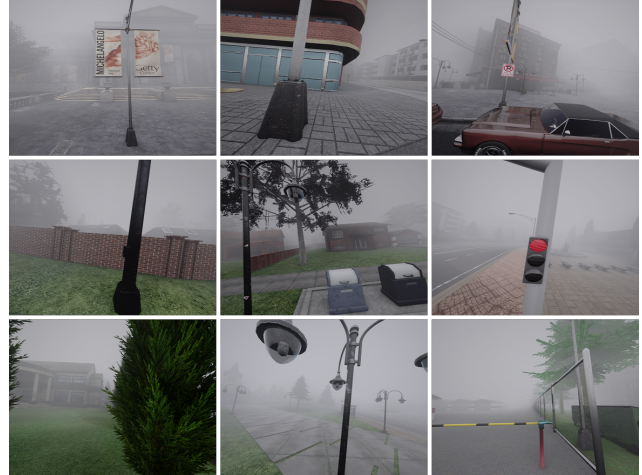
Figure 3. Examples of distance-based haze distribution in CARLA-Haze. Note how objects closer to the camera exhibit higher visual clarity, while distant objects appear increasingly occluded due to atmospheric scattering, despite all scenes having 100% haze intensity.
