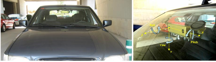
**Fig. 1.** On-board stereo vision sensor with its corresponding coordinate system (right camera coordinate system is used as reference).
