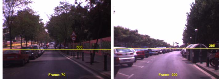
**Fig. 4.** Vanishing lines computed according to the current camera pose—camera height and pitch angle
