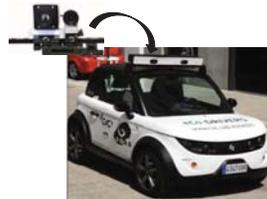
**Fig. 4** Acquisition system (cross-spectral stereo rig on the top left) and electric vehicle used as mobile platform.
