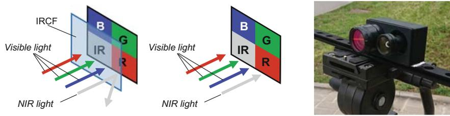
**Fig. 2.** Illustration of: (*left*) infrared filtered imaging system (IRCF: infrared cut-off filter); (*middle*) RGBN imaging system; (*right*) See3CAM-CU4 RGBN cameras used in the experiments. The infrared cut-off filter can be appreciated in the left side of the figure; it is used to generate the ground truth RGB images).
