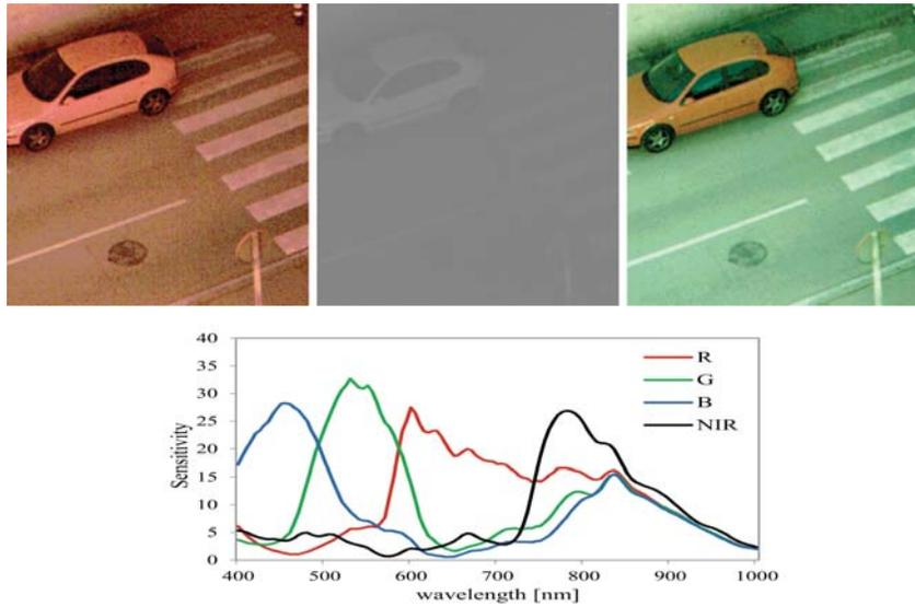
**Fig. 1.** (*top-left*) RGB image (obtained in the spectral band 400–1100 nm) with NIR information overlapped; (*top-middle*) NIR image (400–1100 nm) with RGB information overlapped. (*top-right*) RGB image (400–700 nm) used as ground truth; (*bottom*) Sensor’s spectral sensitivity.
