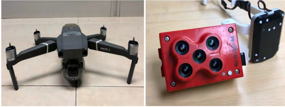
Fig. 2. (left) DJI Mavic 2 Pro-UAV. (right) MicaSense RedEdge-M multispectral camera.
