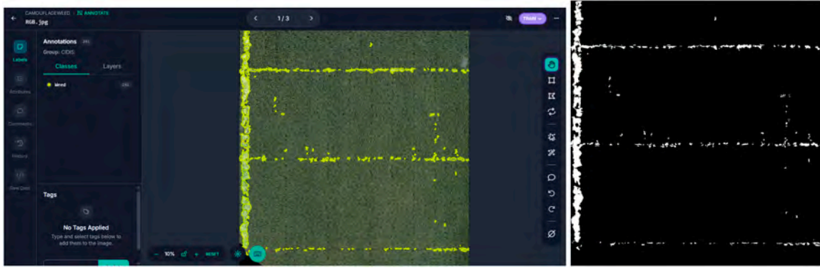
Fig. 5. (Left) View of the Roboflow annotation tool for the RGB orthomosaic image. (Right) Labeled orthomosaic binary mask using Roboflow.
