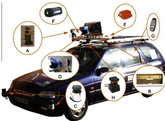
Fig. 12. The ATLASCAR full scale robotic platform. It is equipped with an active perception unit (A), a stereo rig (B), three LRF (C, D, H), a thermal vision camera (F), GPS (G) and an inertial measurement unit (E).
