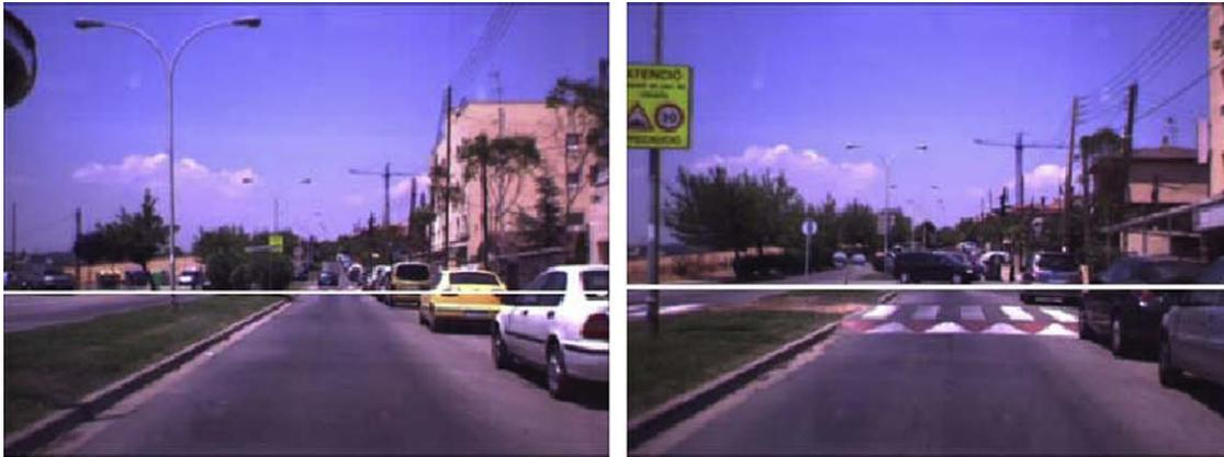
Fig. 8. The estimated horizon line associated with frames 55 and 182 using the road image only.
