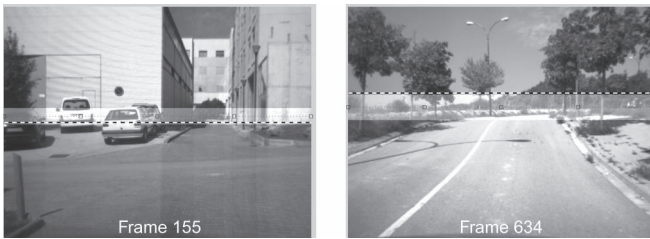
Fig. 11. Frames corresponding to maximum errors between the (brighter image zone highlights the 95% confidence interval of the annotation, whereas dotted-squared lines correspond to the mean value) manually annotated horizon line and (dashed line) automatically computed horizon line. (Left) Cross between roads with different slopes. (Right) Road containing a sharp uphill slope. Notice from the confidence interval that even human evaluation cannot be so accurate in these frames.
