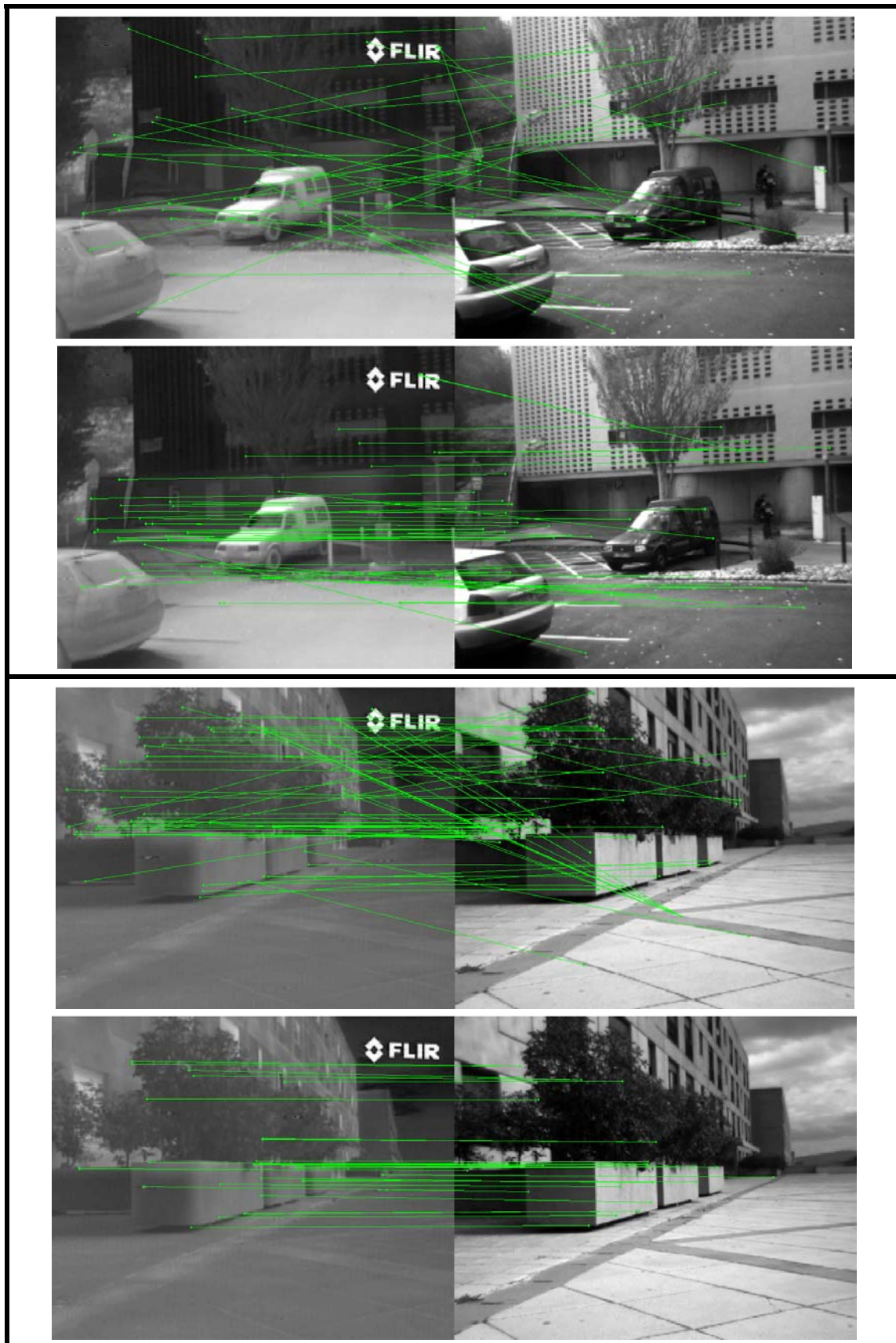
Figure 6. Keypoints matched (green segments) in two image pairs (the whole data set contains 100 pairs of VS-LWIR images) using: (top) SIFT descriptor; (bottom) proposed EOH based descriptor.
