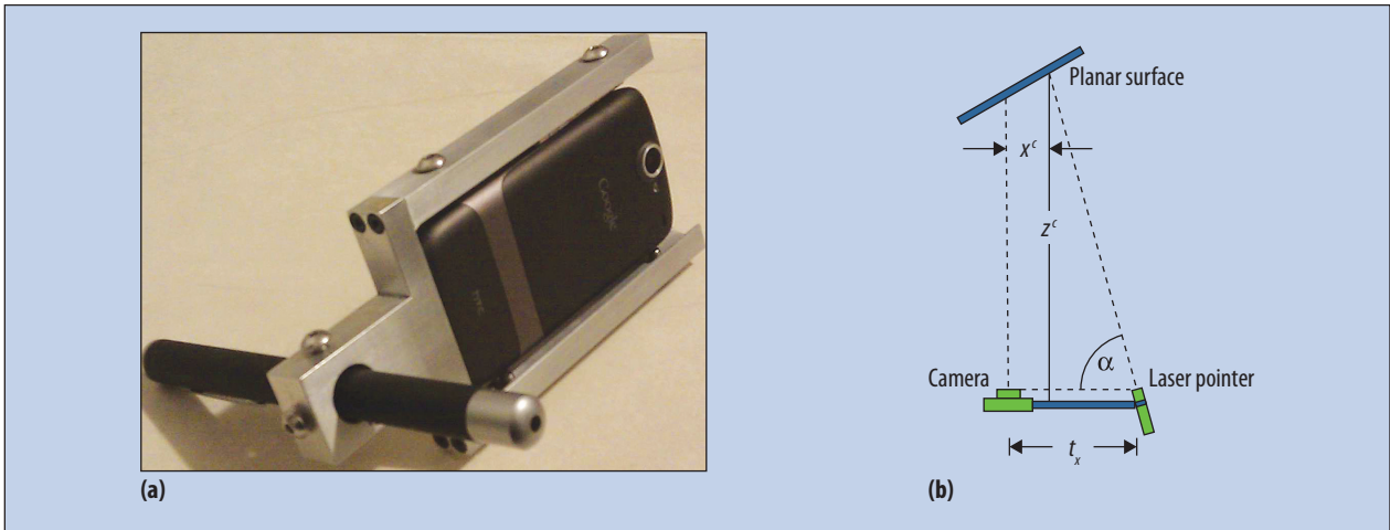
Figure 1. Virtual White Cane. (a) The user carries an Android Smartphone coupled with a laser pointer. The device simulates a white cane vibrating in the presence of obstacles where the user is pointing to. The metallic structure couples the laser pointer and the user's smartphone. (b) As the laser points to an object near the user, a smartphone application uses active triangulation to measure the object's distance ( z^c ) and causes the smartphone to vibrate. As the object gets closer, the vibration intensity increases.
