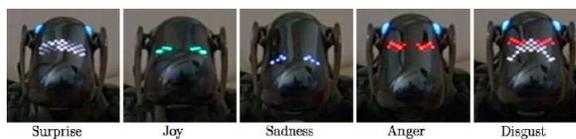
Fig. 7. The figure illustrates the LEDs' configuration for each universal expression.
