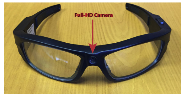
Fig. 2. Smart glasses used as wearable technology. The glasses have embedded in them a high-definition camera in the bridge connecting the two lenses.
