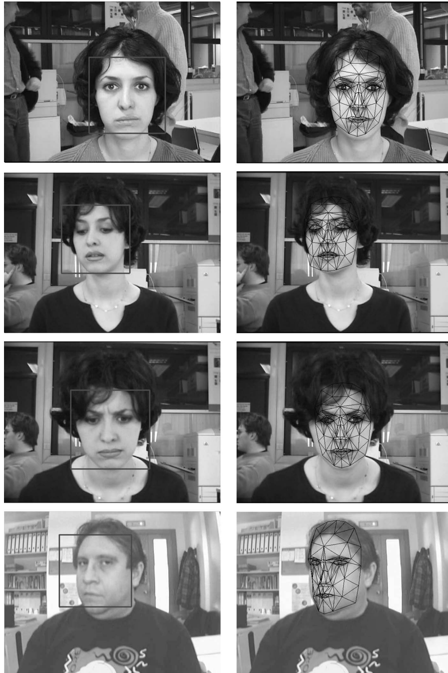
Fig. 6. Automatic 3-D head-pose initialization. (Left column) Four unseen images together with the 2-D face detector results. (Right column) Corresponding estimated 3-D head-pose using the DE algorithm.
