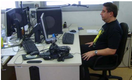
Figure 8. The experimental setup. The camera (in this image placed between the monitor and the keyboard) perceives user's 3D head pose and transmits it to the robot.
