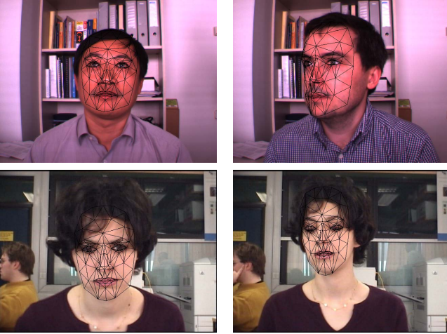
Figure 5. Single snapshot-based initialization of the 3D head pose and face shape parameters associated with three different persons.
