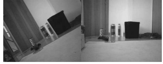
Fig. 6. Correct view matching despite image rotation
