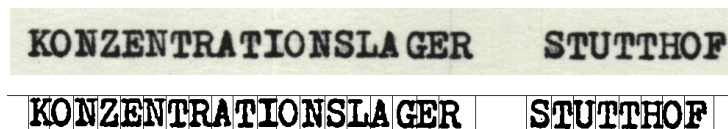
Fig. 4. A field in a catalogue card and the corresponding result after character location and enhancement.
