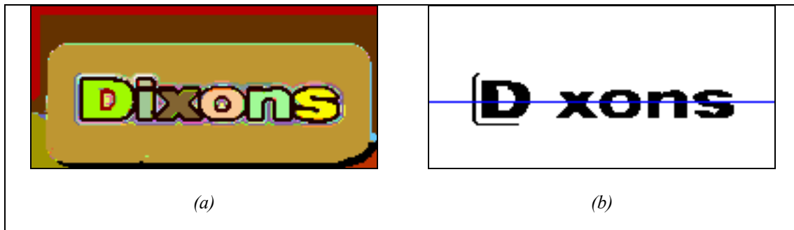
Figure 7-31 – (a) A segmentation produced with the Split and Merge method. A number of components associated with the outlines of the characters can be seen. (b) One of the text lines extracted. A non-character component is erroneously classified as text.
