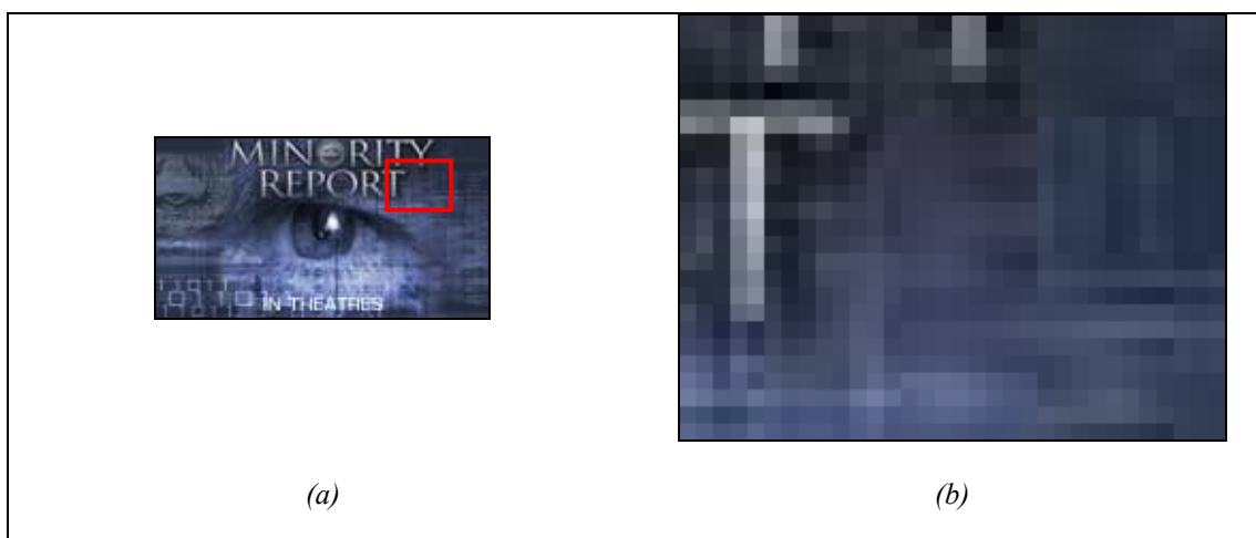
Figure 1-7 – (a) A JPEG compressed image. (b) Magnified part of the image. The block structure produced by JPEG compression is visible in large areas, while more compression artefacts are visible near the characters.
