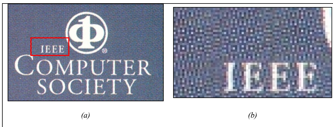
Figure 8-1 – (a) Part of a scanned magazine cover. (b) Magnified region, where dithering is visible.
