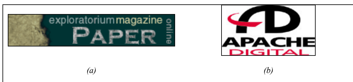
Figure 7-5 – (a) An image belonging to category A (multicoloured text and background). The number of colours used in this image is only 64. (b) An image belonging to category D (single-colour text and background). The number of colours in this image is 1,973, mainly due to antialiasing.
