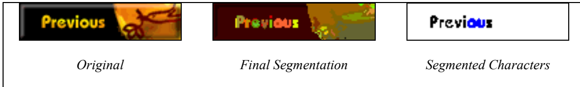
Figure 4-29 – Image containing single-coloured background and multi-coloured text. Anti-aliasing produces a fuzzy area between characters “o” and “u” that ultimately causes the merging of the characters.
