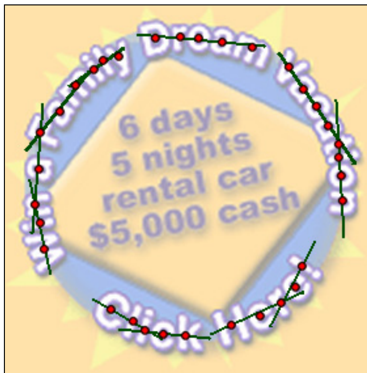
Figure 6-12 – Straight lines fitted on circularly written text. The centres of gravity of the character components are shown in red and the lines fitted in dark grey. As can be seen, many of the lines comprise a small number of components because of the way text is written.
