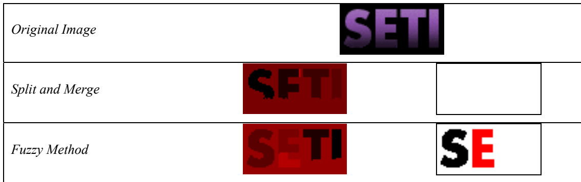
Figure 7-28 – An example of an image with gradient text. The Split and Merge method merges parts of the character with the background.
