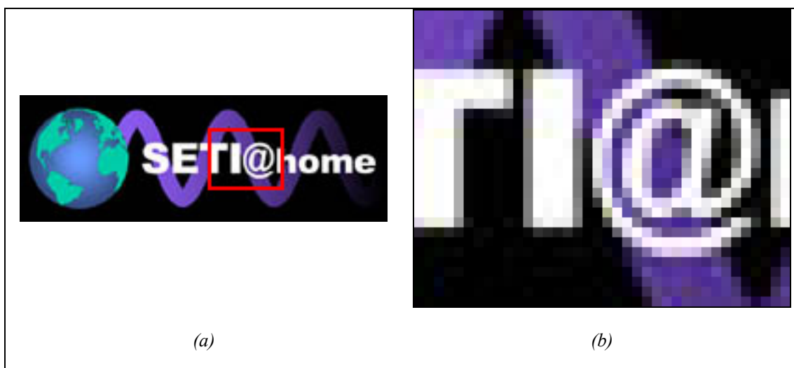
Figure 1-4 – (a) An image with antialiased characters. The area marked with the red rectangle appears in magnification on the left. (b) Magnified part of the image, where the antialiased edges of characters are visible.
