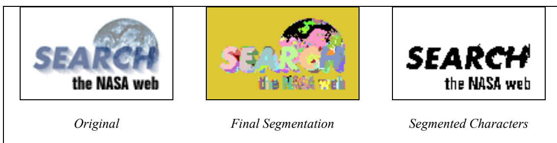
Figure 4-31 – Results for the same image as in Figure 4-28, using stricter lightness thresholds. In this case, letter “E” is identified, and letter “w” is not broken into smaller components.
