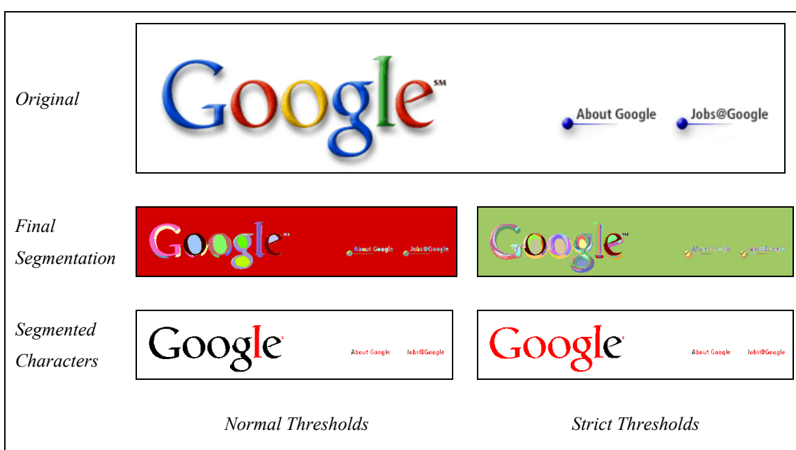
Figure 4-32 – An image with multi-coloured characters. Because a number of shades of the same colour are found in each character, using stricter lightness thresholds prevents the method from identifying each character as a whole component.
