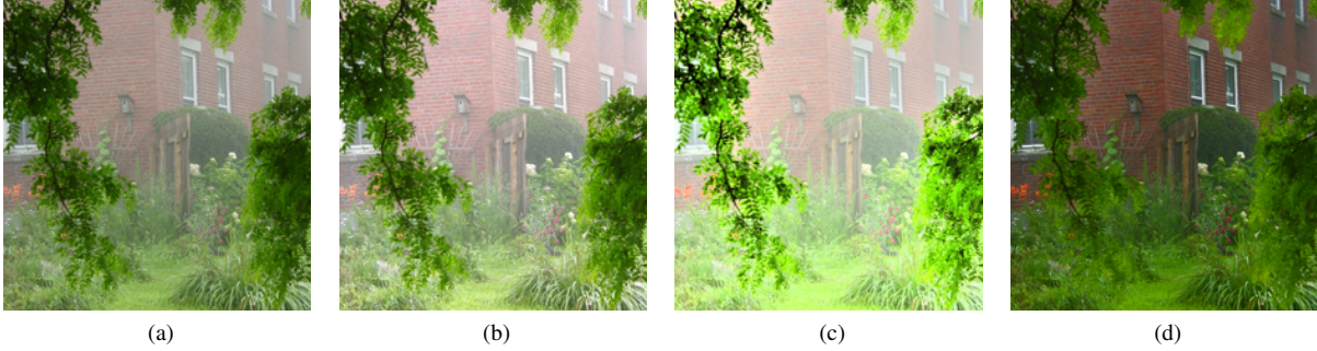
Figure 2: Retinex cannot decrease brightness. (a) Hazy image (b)-(d) Output of: (b) Random Spray Retinex [35] (c) Multi-Scale Retinex [18] (d) Multi-Scale Retinex used for image dehazing, following eq. (1).
