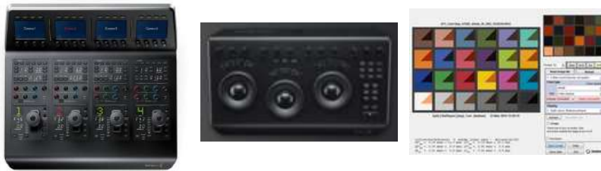
Figure 7.2: On the left, a camera control unit; on the middle, the DaVinci Resolve tool; and on the right, the Imatest software for colour correction based on colour charts. Images from [Design, 2018] and [Imatest, 2018].
