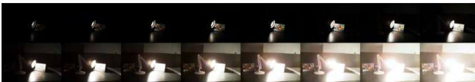
Figure 5.2: Sixteen individual exposures used by M. Fairchild in [Fairchild, 2007] to create the LuxoDoubleChecker HDR image. Figure adapted from [Fairchild, 2007].
