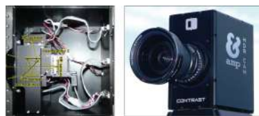
Figure 4.7: Camera prototype from [Tocci et al., 2011]. On the left the optical set-up, and on the right the camera final prototype. Image from [Tocci et al., 2011].
