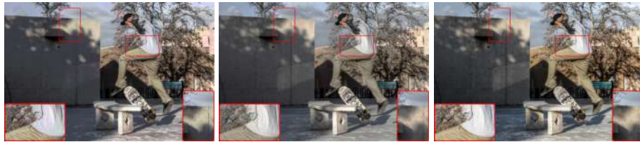
Figure 5.11: HDR results on a dynamic scene applying the HDR creation method of Sen et al. [Sen et al. , 2012] with three different linearisation techniques: Debevec and Malik [Debevec and Malik, 1997] (left), Lee et al. [Lee et al. , 2013] (middle), and Step 1 of our proposed method (right), taking as reference the image in the mid-point of the sequence. HDR results tone-mapped with Mantiuk et al. [Mantiuk et al. , 2008].
