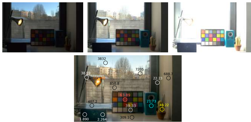
Figure 1.1: On top row, images acquired with different exposure times using a Nikon D3100, from [1/160, 1/10, 1.6]. The image on the bottom row corresponds to the reconstructed HDR image from the set above. For display purposes, the image has been tone-mapped.
