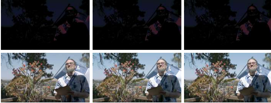
Figure 6.12: Top row: frames from a dual-ISO video. Bottom row: results obtained with proposed method. The video does not show temporal artifacts.
