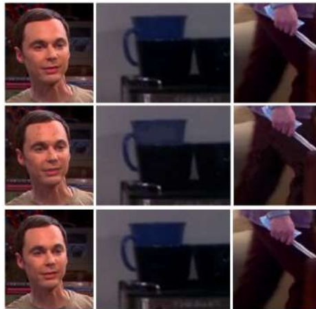
Figure 5.14: Spatial artifacts due to GRA-RGB. Top row: original images. Middle row: effect of extreme target gamut. Bottom row: effect of realistic target gamut. The relationship of target gamut and spatial artifacts can be seen at the forehead of the person, cup and on the pants.
