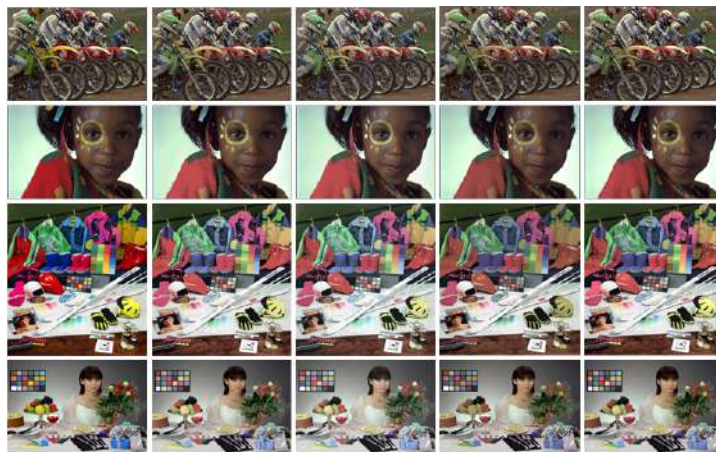
Figure 5.9: Results of GRAs on still images. Column 1: original images. Column 2: output of HPMINDE [Murch and Taylor, 1989]. Column 3: output of [Lau et al., 2011]. Column 4: output of [Alsam and Farup, 2012]. Column 5: output of our GRA-RGB.
