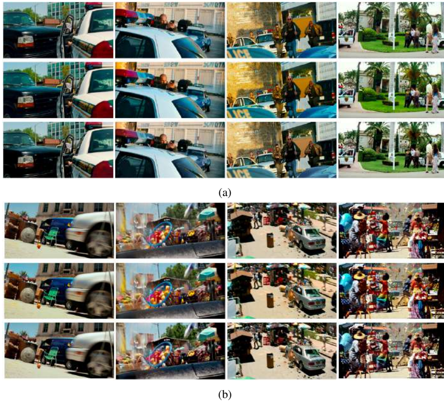
Figure 5.17: Results of GEAs. (a) Image sequence 1. (b) Image sequence 2. In both image sequences; top row, ground truth (BT.709 gamut); middle row, output of Same Drive Signal algorithm [Laird et al., 2009]; bottom row, output of our GEA. In both image sequences, the results of our GEA are more pleasing and perceptually faithful to the ground truth as compared with the output of the SDS algorithm [Laird et al., 2009]; see zoomed-in details in Fig. 5.18. Both image sequences are the property of Paramount Pictures and taken from [Pictures, 2013].
