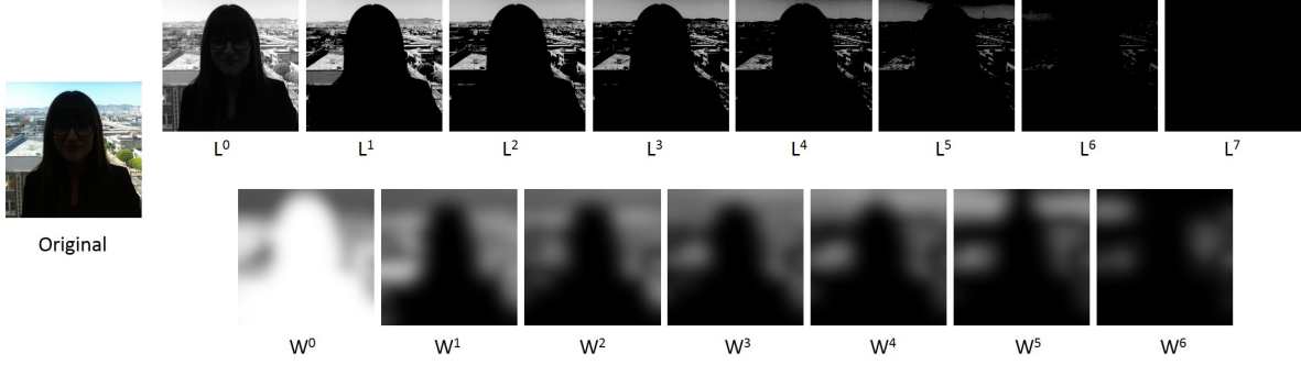
Figure 1. Original image (left), the iterates from the gradient descent (top) and the weight maps associated to these iterates (bottom).
